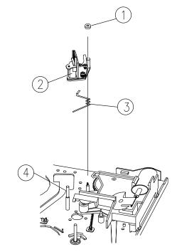
Fig.3-10 DISASSEMBLY OF THE AC HEAD ASS'Y
